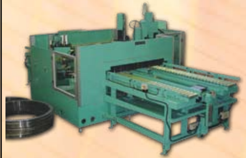
Example 3 – Large (6 ft) gear ring 2-sided chamfering with conveyor feed system
