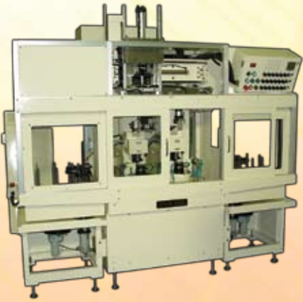
Example 1 – Dual spindle, dual cutting head with part magazine and automatic loading/unloading
