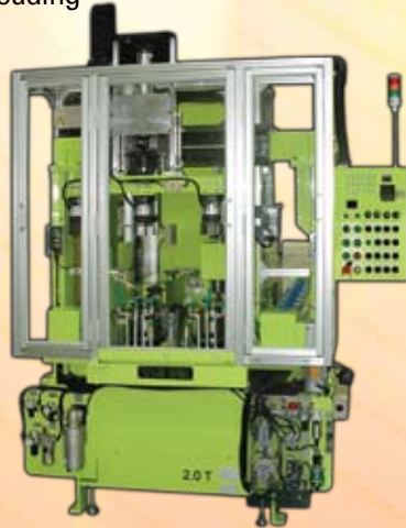
Example 2 – Dual spindle, dual cutting head with conveyor and auto loading/unloading
